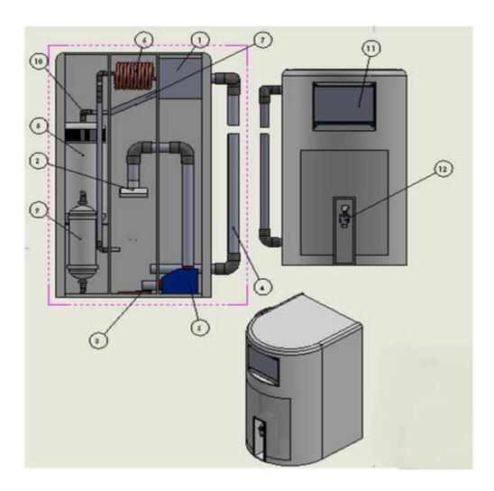
Fig. Distillation based water purification system
